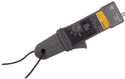
Figure 2 Connection between the Test Clamp and Conductor
